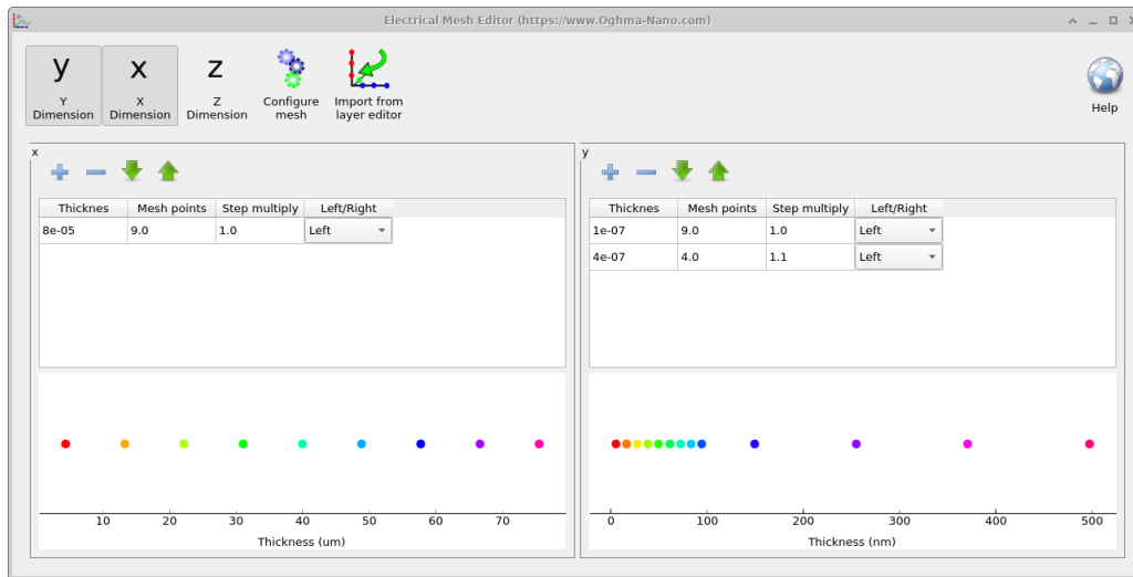
Figure 8.3: The electrical mesh editor showing the mesh for a 2D OFET simulation.
